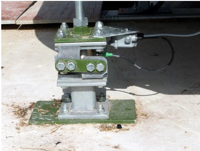
Fig. 6: Weighing foot with integrated load cell; amplifier mounted on weighing foot
