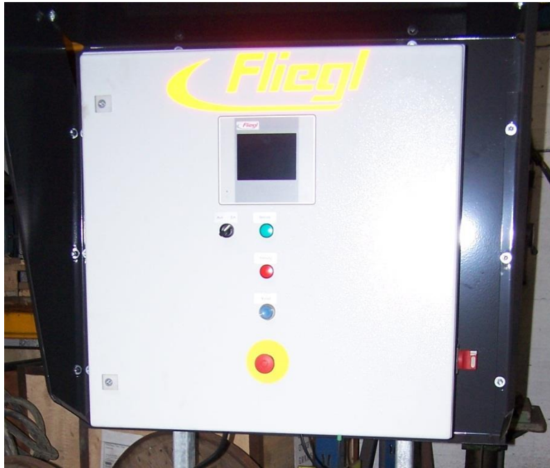
Fig. 1: Control system switchgear cabinet - "DigiTouch Bio" as a control system
