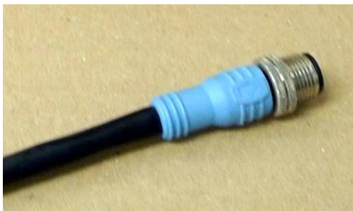
Fig. 21: Blue – bus signals such as CAN bus and RS485
