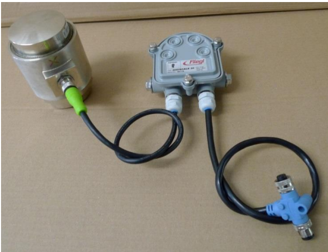
Fig. 5: Analogue load cell with external amplifier
